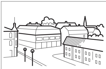
Terrain Type III Area covered with vegetation or buildings or with some obstacles with largest mutual distance equal to 20 times the height of obstacles (eg villages, suburbs, woodland).
